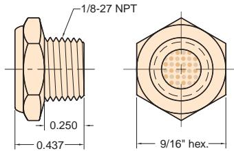
**Material:** Solid brass body; sintered stainless steel insert (100 micron)
